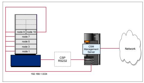
Figure 1-1 Frame with nodes managed by CSM
