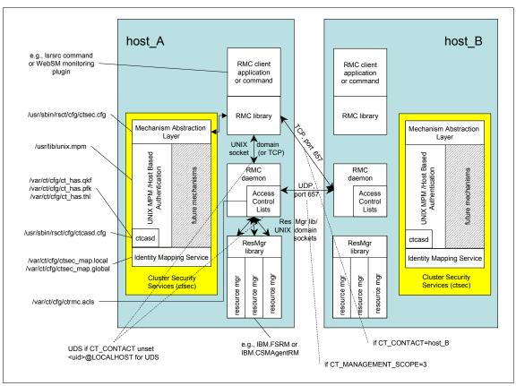
Figure 7-5 RSCT communication flow
