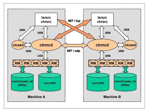
Figure 4-2 RSCT's distributed RMC architecture.
