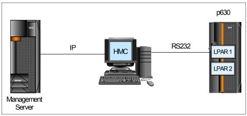
Figure 1-3 A p630 with two LPARs in a Cluster 1600 managed by CSM
