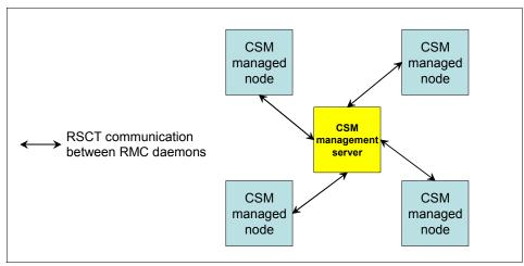
Figure 7-4 RMC communication in a CSM management domain
