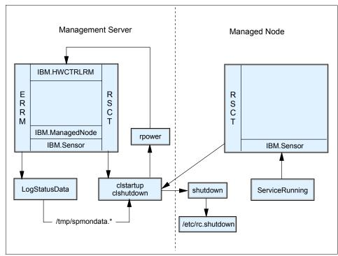
Figure B-1 Cluster startup/shutdown architecture diagram
