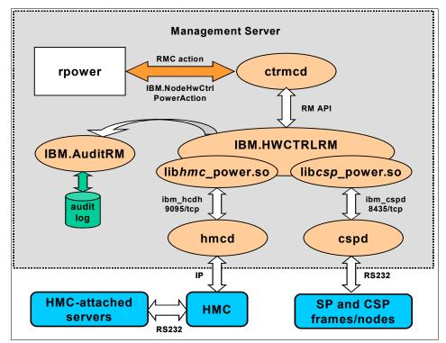
Figure 5-4 CSM hardware control subsystem
