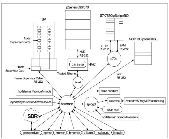
Figure 5-3 SP hardware control in PSSP
