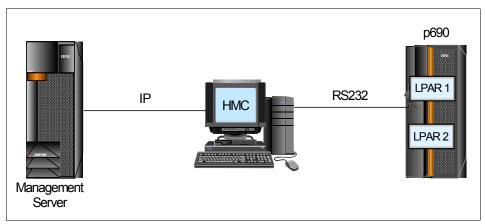
Figure 1-2 p690 with two LPARs in a Cluster 1600 managed by CSM
