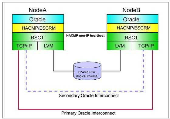
Figure 2-1 HACMP and RAW devices configuration
