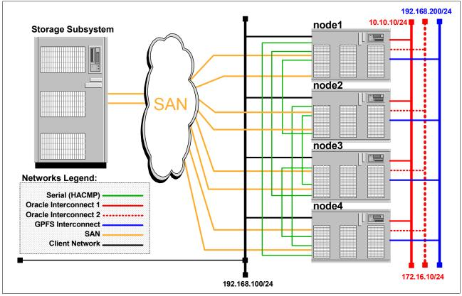
Figure 3-1 Hardware architecture
