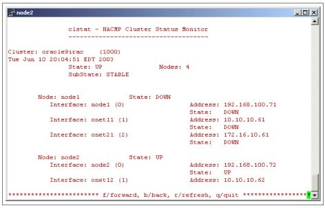
Figure 3-44 clstat -a command output
