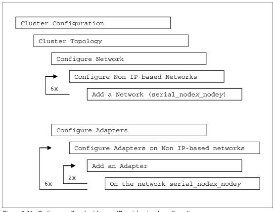
Figure 3-11 Smit menus flowchart for non-IP serial network configuration
