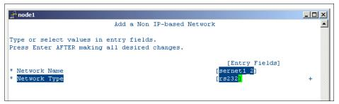
Figure 3-36 Entering the characteristics of the serial network
