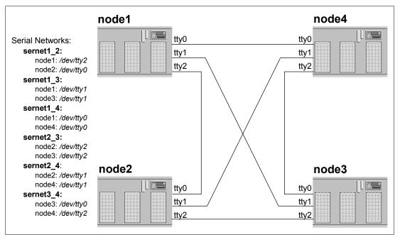
Figure 3-29 shows the serial network topology based on a 4-node cluster.
