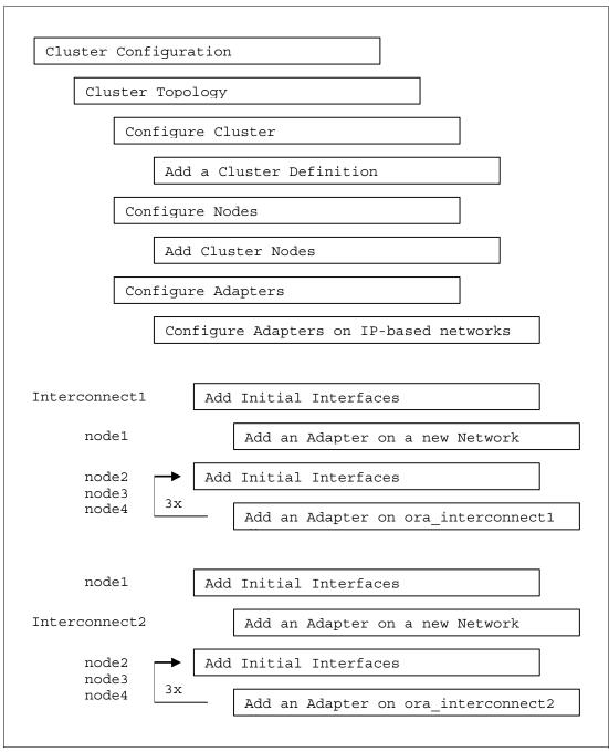
Figure 3-10 Smit menus flowchart for cluster node and interconnect network configuration
