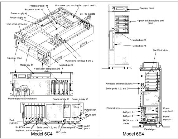
Figure 1-6 Views of pSeries 630 models 6C4 and 6E4<sup>8</sup>
