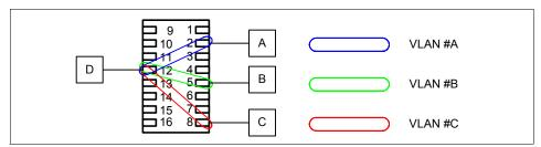
Figure C-4 Overlapping port definition based on the port-based VLAN
