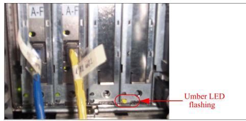
Figure 11-22 Umber LED flashing in a PCI slot
