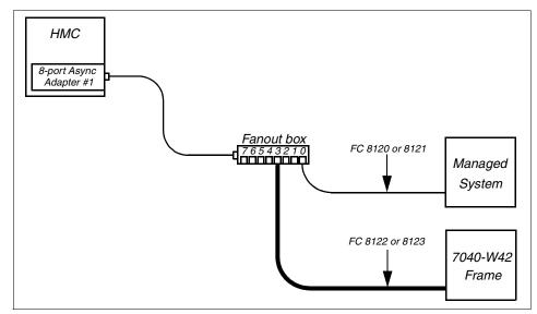
Figure 1-13 Connecting with an 8-port asynchronous adapter
