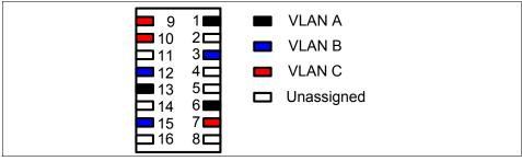
Figure C-3 Port-based VLAN concept
