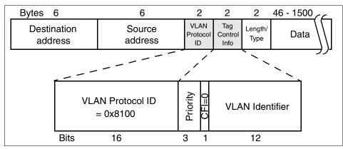
Figure C-5 VLAN-tagged Ethernet frame
