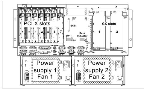
Figure 1-5 Rear view of pSeries 650 Model 6M2
