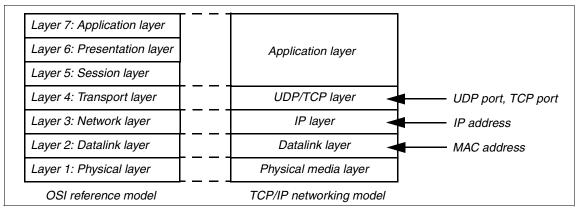
Figure C-1 OSI seven-layered networking reference model and TCP/IP model
