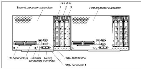
Figure 1-4 Rear view of pSeries 655<sup>7</sup>
