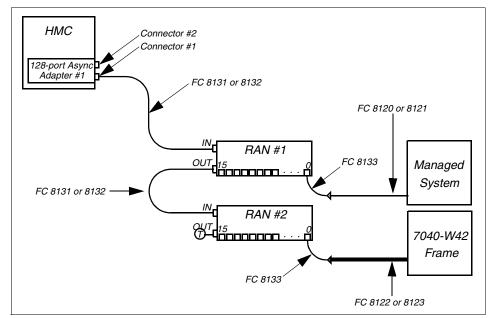
Figure 1-14 Connecting with a 128-port asynchronous adapter
