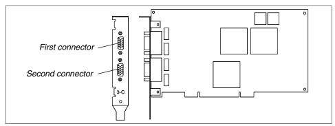
Figure 1-15 128-port asynchronous adapter card edge
