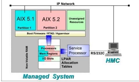
Figure 1-2 Communication between the HMC and the service processor
