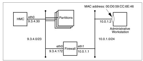
To show how IP filtering can be set up between the administrative workstation and HMC, we have configured the sample network configuration in Figure 8-6.
