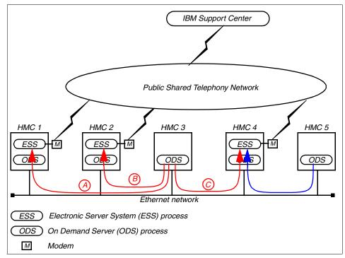
Figure 11-10 Service Agent client/server configuration on multiple HMCs
