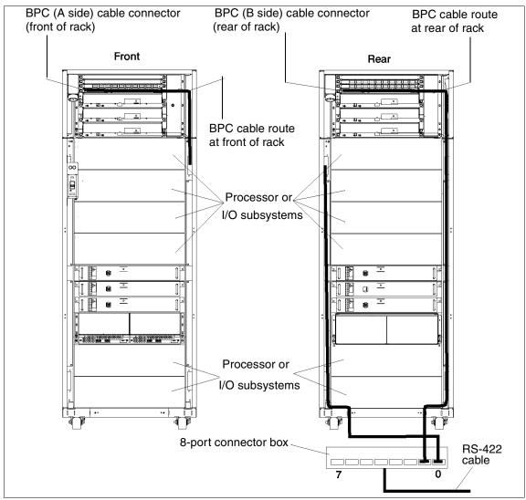
Figure 1-8 RS-422 serial cable connection from HMC to 7040-W42 system rack<sup>10</sup>
