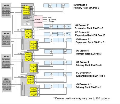
Figure B-7 Configuration for maximum number of adapters and disks
