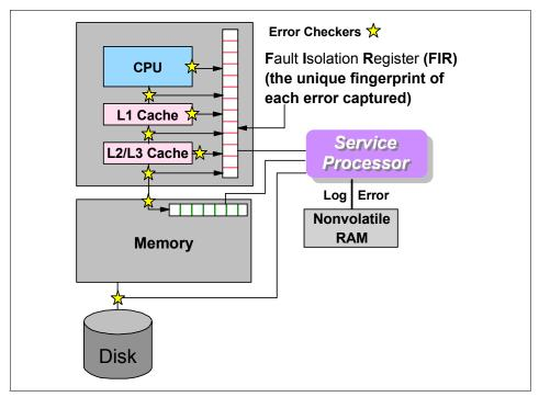
Figure 5-2 FFDC error checkers and fault isolation registers
