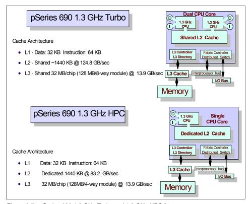
Figure 2-7 pSeries 690 1.3 GHz Turbo and 1.3 GHz HPC feature
