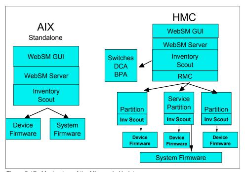
Figure 5-17 Mechanism of the Microcode Updates
