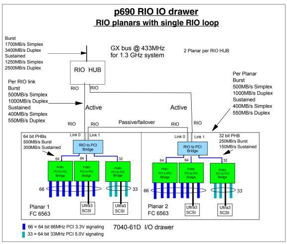
Figure B-1 RIO drawer, in single-loop mode on a 1.3 GHz server
