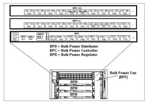
Figure 2-31 Power subsystem locations in BPA
