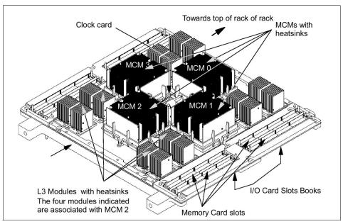
Figure 2-4 CEC backplane orthogonal view
