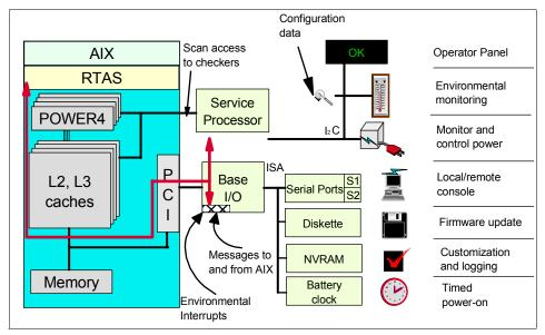
Figure 5-1 Service processor schematic
