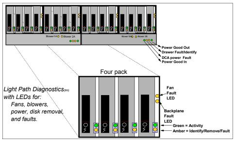
Figure 5-8 Status LEDs for components in I/O drawers
