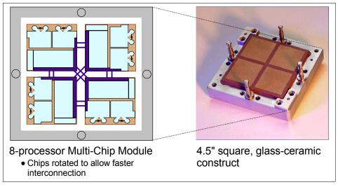
Figure 2-5 POWER4 multichip module
