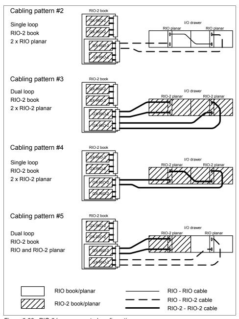
Figure 2-22 RIO-2 loops supported configurations
