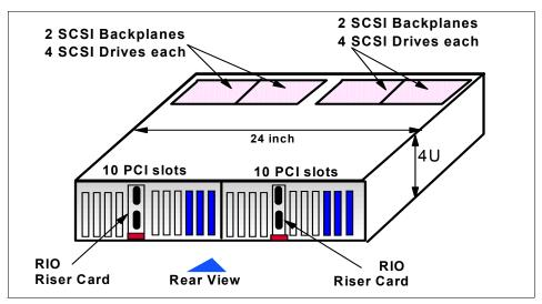
Figure 2-17 I/O drawer rear view
