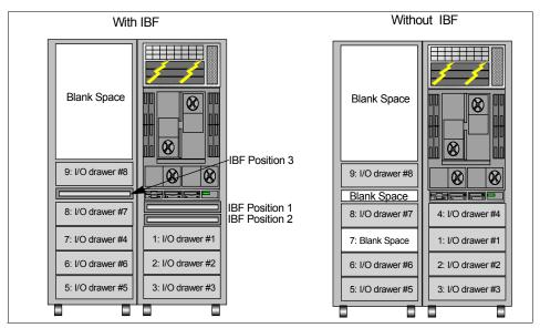
Figure 2-25 I/O drawer and IBF placement positions (pSeries 690)
