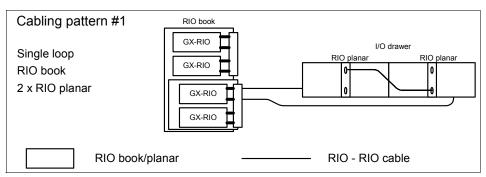
Figure 2-21 RIO loops supported configurations
