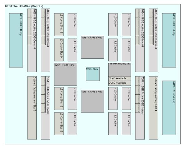
Figure 3-7 Detailed diagram for the pSeries 690 CEC
