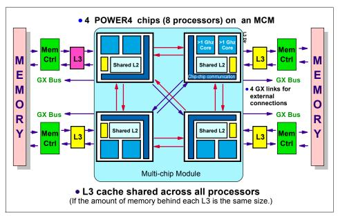
Figure 2-6 Multichip module with L2, L3, and memory
