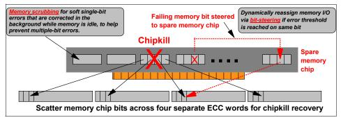
Figure 5-3 Memory error recovery mechanisms
