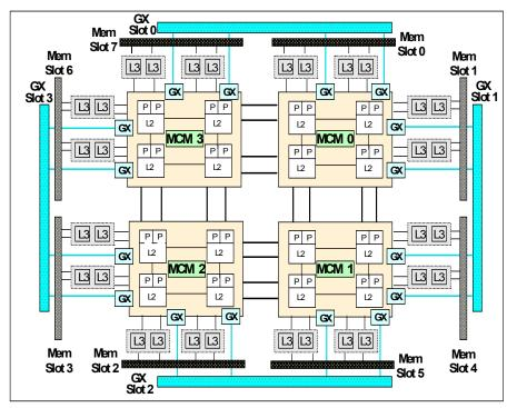
Figure 2-9 Logical relationship between MCMs, memory, and GX Slots
