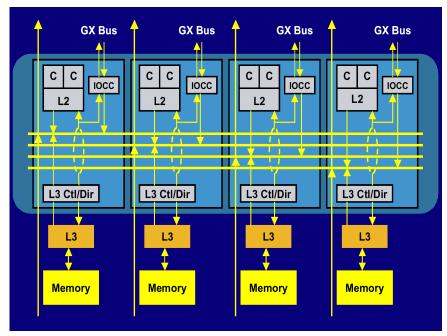
Figure 2-11 Interconnection between processors in an MCM
