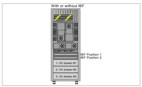
Figure 2-26 I/O drawer and IBF placement positions (pSeries 670)
