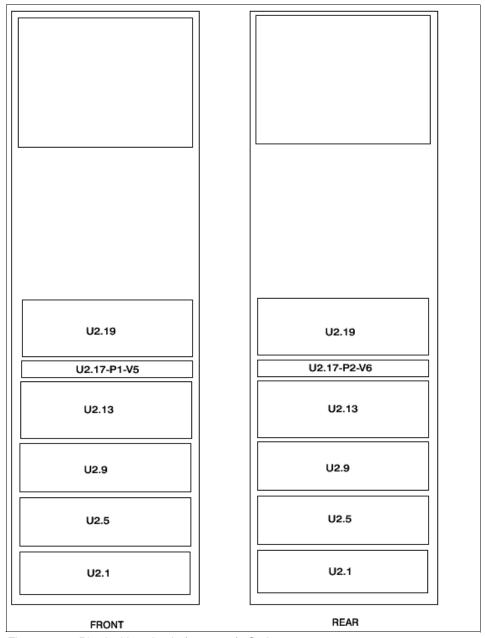
Figure 2-28 Physical location in frame 2 of pSeries 690
