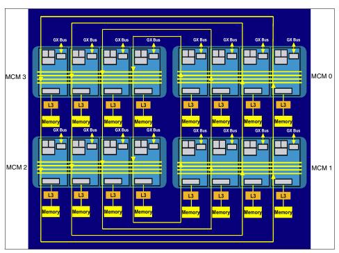
Figure 2-10 Interconnection between four MCMs
