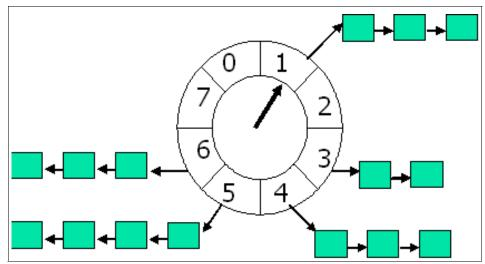
Figure 6-1 shows a simplified model of a timer-wheel algorithm.
