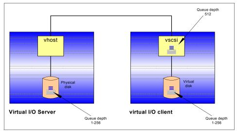
Figure 5-1 Physical disk mapped to a virtual disk
