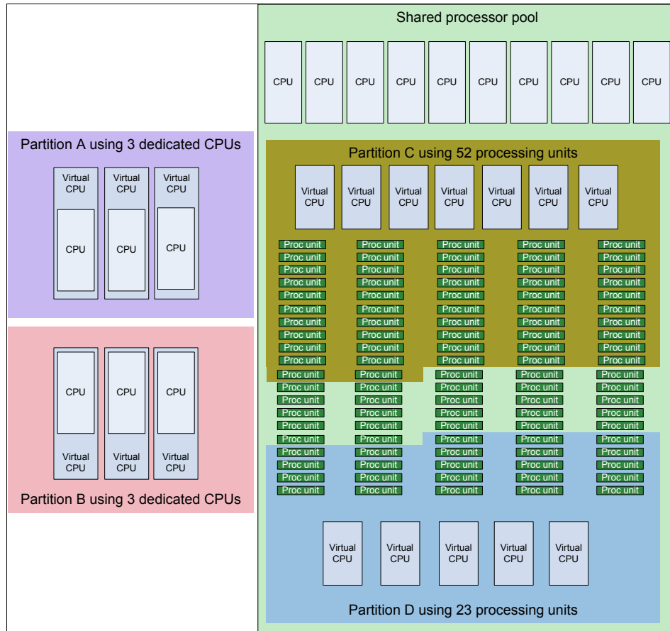
Figure 14-1 16-core system with dedicated and shared CPUs
