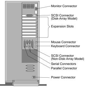
*Note:* Some Micro Channel models come with a preinstalled PeerMaster adapter in a Micro Channel expansion slot.
