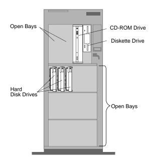
**Open Bays:** Your server has a special design that gives you the flexibility to use up to 18 hot-swap, 3.5-inch hard disk drives. There is additional open space in the top left bay for two more diskette drives or an additional SCSI drive. For installation instructions and information on the types of drives that you can install in each bay, see your *User's Handbook*.
