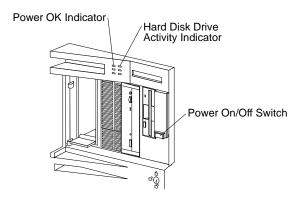
**Power On/Off Switch:** Press this to turn your server on or off. Do not turn off your server if any drive activity indicator is on. This might damage the information stored on a hard disk or diskette.
