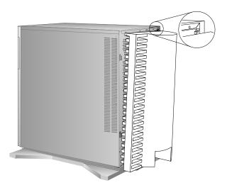
The security-cover option prevents the cables from being removed from the rear of the server, and prohibits other computers or devices from being attached to the unused connectors.
