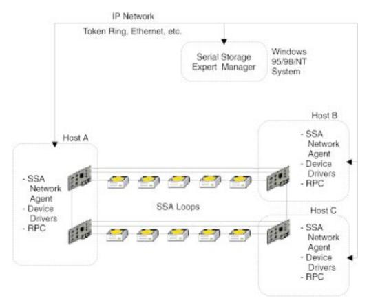
Figure 1. IBM StorWatch Serial Storage Expert - Overview
