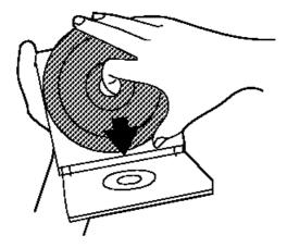
5. Close the caddy, and with the arrow pointing toward the CD-drive slot, insert caddy in the slot.
