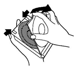
4. Insert the CD-ROM disc into the caddy. The printed side of the disc faces the transparent cover.
