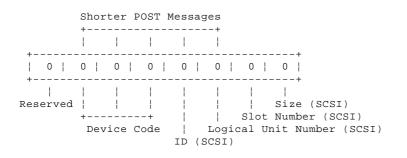
All SCSI devices must be set to a different SCSI ID. Duplicate SCSI ID settings can generate a false error message. Use the SCSI ID to determine whether the error message is coming from an internal or an external device.
