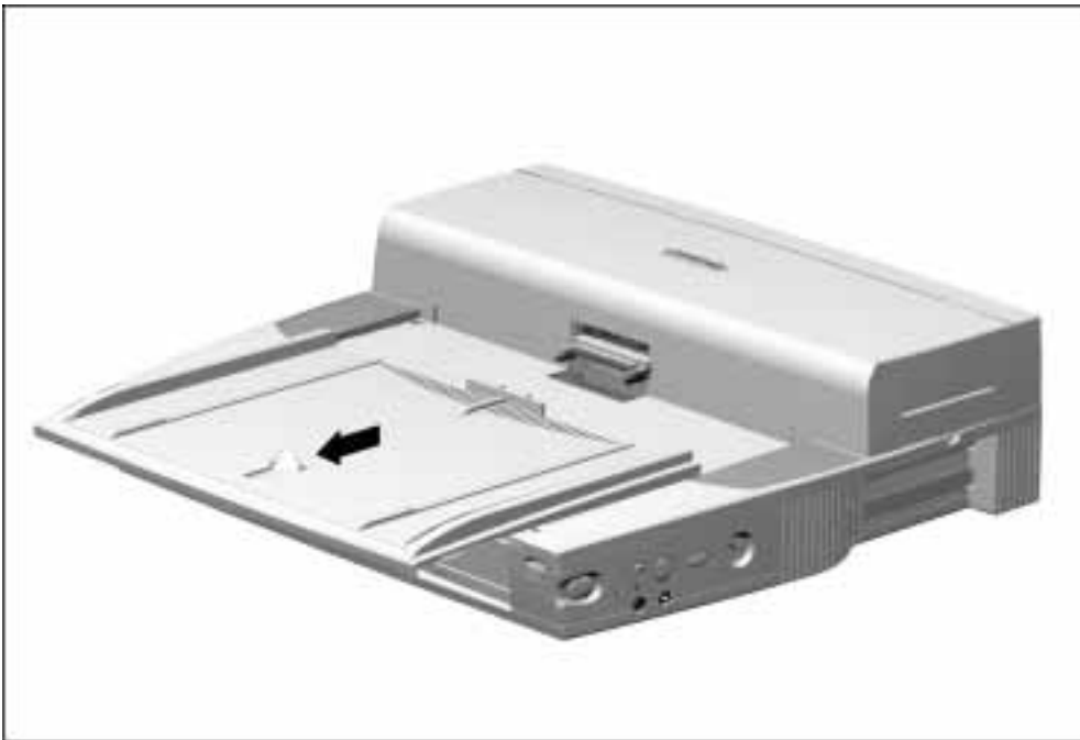
Figure 5-6. Removing the Alignment Tray Assembly
