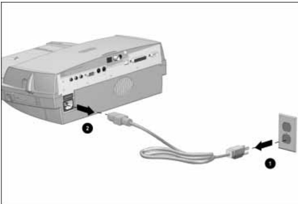
Figure 6-3. Disconnecting the Armada MiniStation
