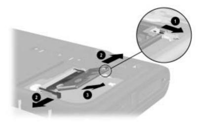
Figure 5-13. Removing a Mini PCI Communications Board
