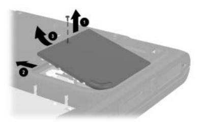
*Figure 5-12. Removing the Mini PCI Communications Slot Cover*
