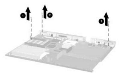
Figure 5-44. Removing the System Board Screws
