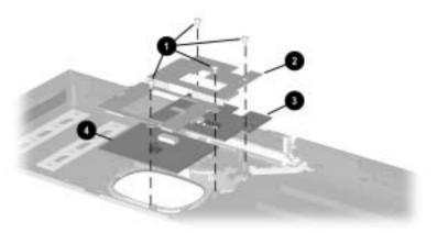
*Figure 5-33. Removing the TouchPad Components on TouchPad Models*
