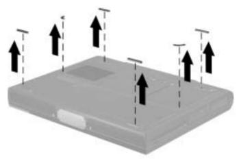
Figure 5-9. Replacing the Computer Feet
