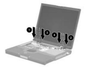
Figure 5-26. Installing the Display Screws
