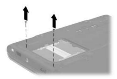
Figure 5-4. Removing the Optical Drive Screws
