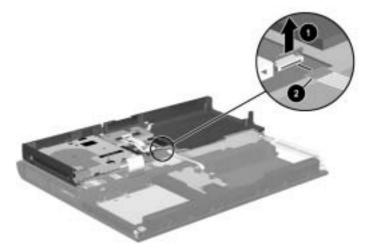
Figure 5-29. Disconnecting the Keyboard-to-TouchPad Cable
