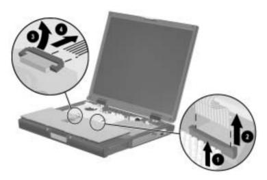
Figure 5-19. Disconnecting the Keyboard-to-TouchPad Cable
