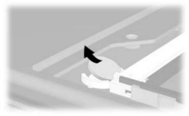
Figure 5-14. Removing the Disk Cell RTC Battery
