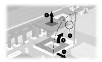
Figure 5-22. Removing the Processor
