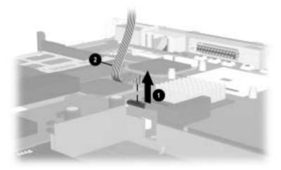
Figure 5-41. Removing the System Board-to-TouchButton Board Cable
