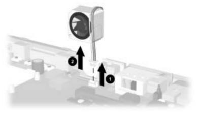
Figure 5-42. Removing the Fan
