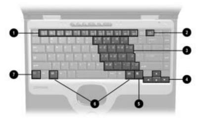
Figure 1-4. Keyboard Components
