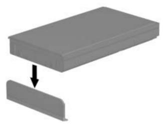
Figure 5-3. Removing the Battery Bezel
