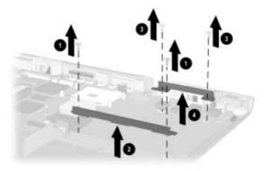
Figure 5-43. Removing the Optical Drive Alignment Rails
