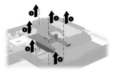
Figure 5-37. Removing the Charger Board
