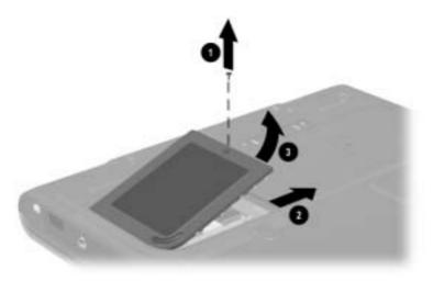
*Figure 5-10. Removing the Memory Expansion Compartment Cover*
