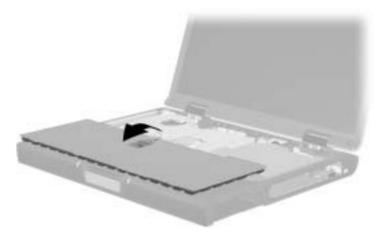
Figure 5-18. Releasing the Keyboard
