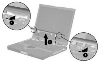
Figure 5-17. Removing the LED Cover
