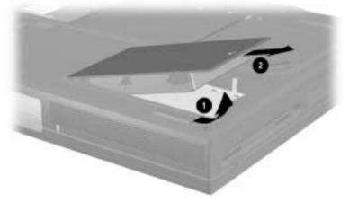
Figure 5-7. Removing the Hard Drive
