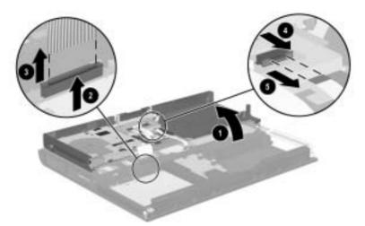
Figure 5-28. Removing the Palm Rest
