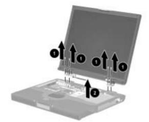
Figure 5-24. Removing the Display
