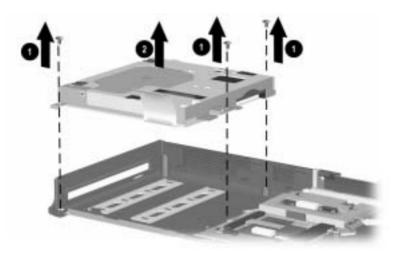
Figure 5-30. Removing the Diskette Drive
