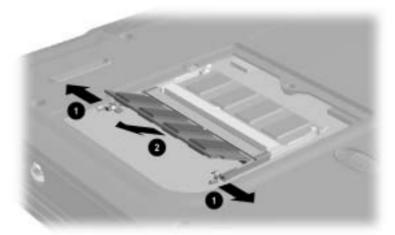
Figure 5-11. Removing a Memory Expansion Board
