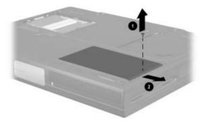
Figure 5-6. Removing the Hard Drive Screw
