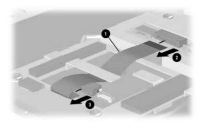
Figure 5-32. Removing the TouchPad-to-TouchButton Board Cable
