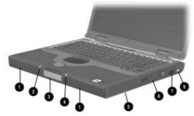
Figure 1-2. Front and Right Side Components
