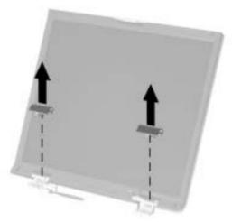
Figure 5-25. Removing the Display Hinge Covers
