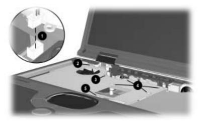
Figure 5-20. Removing the Heat Spreader Screws
