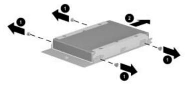
Figure 5-8. Removing the Hard Drive Bracket
