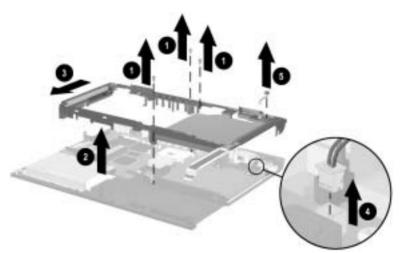
Figure 5-40. Removing the Top Cover and Microphone
