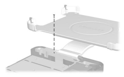
Figure C-12. Phillips M2.5 x 12.0 Screw Location
