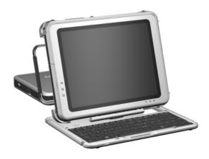
Figure 1-2. Compaq Tablet PC TC1000 with Optional Keyboard and Optional Docking Station
