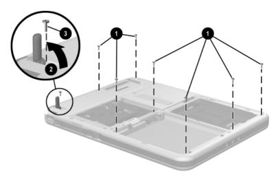
Figure 5-9. Removing the Display Panel Assembly Screws
