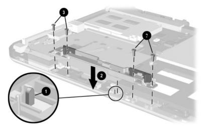
Figure 5-21. Installing the Keyboard Release Assembly
