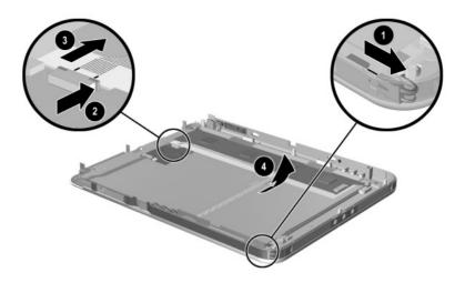
Figure 5-13. Disconnecting the Display Panel Cables
