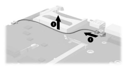
Figure 5-28. Removing the Modem Cable
