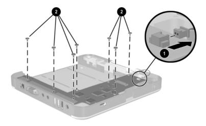
Figure 5-34. Removing the Board Assembly Screws
