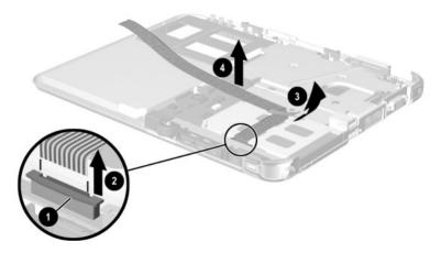
Figure 5-18. Removing the Speaker Cable
