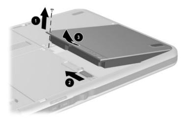
Figure 5-2. Removing the Battery Pack
