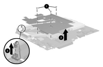
Figure 5-26. Removing the EMI Shield
