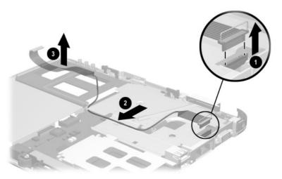
Figure 5-19. Removing the Digitizer Cable
