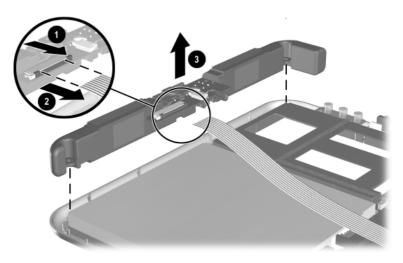
Figure 5-17. Removing the Speaker Assembly
