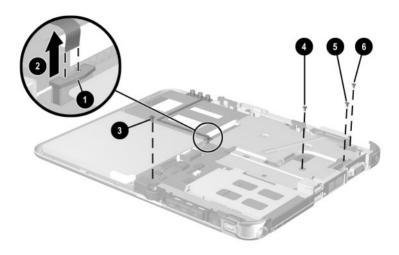
Figure 5-24. Removing the System Board Screws
