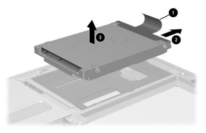
Figure 5-7. Removing the Hard Drive
