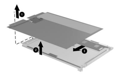
Figure 5-15. Removing the Digitizer
