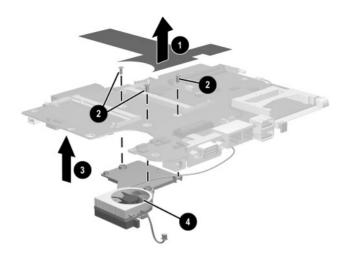
Figure 5-27. Removing the Fan and Heat Sink
