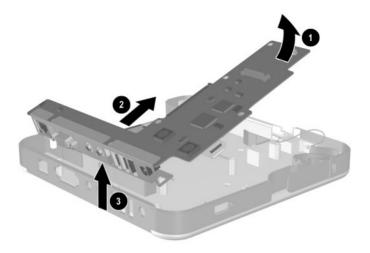
Figure 5-35. Removing the Board Assembly
