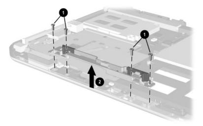
Figure 5-20. Removing the Keyboard Release Assembly
