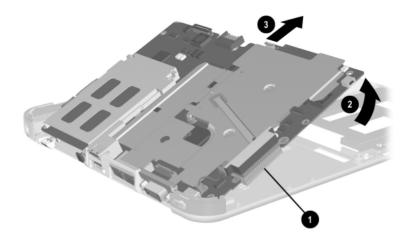
Figure 5-25. Removing the System Board
