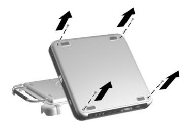
Figure 5-30. Removing the Top Case Screws
