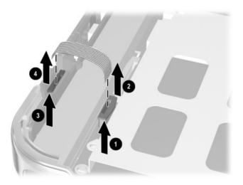
Figure 5-23. Removing the Switch Board Cable
