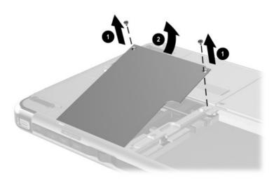
Figure 5-3. Removing the Memory Expansion/Mini PCI Communications Compartment Cover
