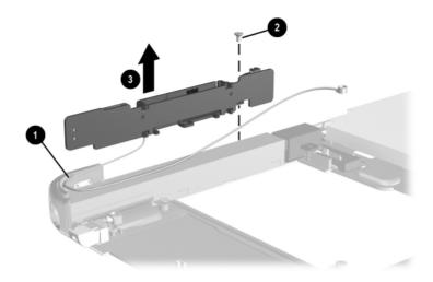
*Figure 5-29. Removing the Switch Board*Reverse the preceding procedures to install the switch board.
