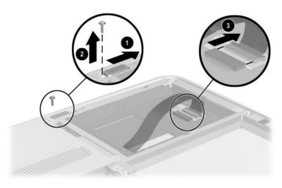
Figure 5-10. Removing the Display Panel Assembly Screw and Disconnecting the Digitizer Cable
