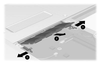
Figure 5-5. Removing the Memory Expansion Board
