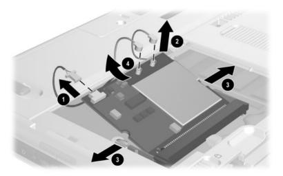
Figure 5-4. Removing the Mini PCI Communications Board
