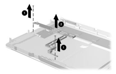
Figure 5-12. Removing the Display Panel Bracket
