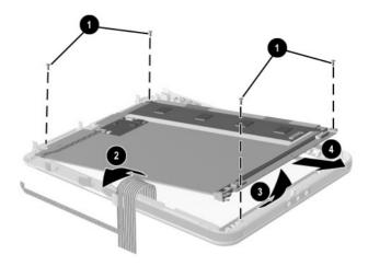
Figure 5-14. Removing the Display Panel
