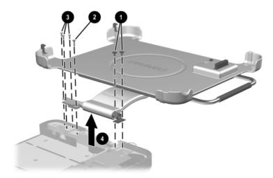
Figure 5-33. Removing the Docking Stand and Pivot Arm
