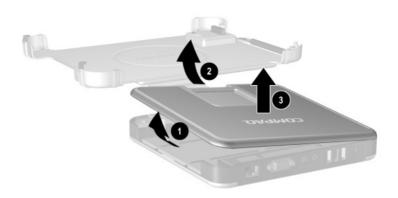
Figure 5-31. Removing the Top Case
