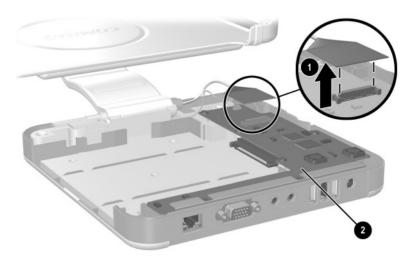
Figure 5-32. Disconnecting the Docking Stand Cable
