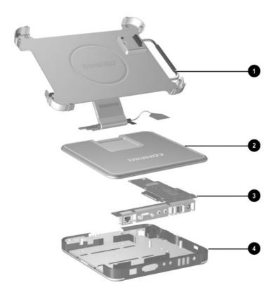
Figure 3-7. Compaq Tablet PC TC1000 Docking Station Components
