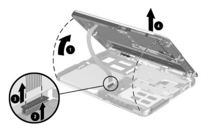
Figure 5-11. Removing the Display Panel Assembly
