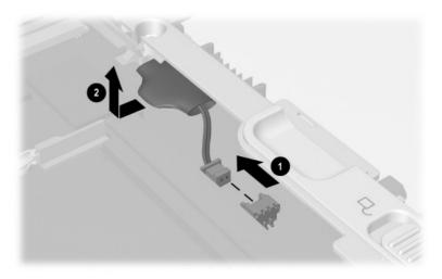
Figure 5-8. Removing the RTC Battery
