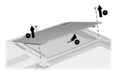
Figure 5-6. Removing the Hard Drive Cover
