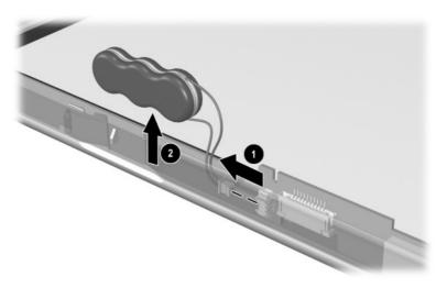
Figure 5-16. Removing the Bridge Battery
