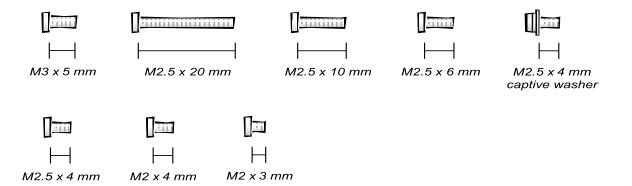
NOTICE: When reinstalling a screw, you must use a screw of the correct diameter and length. Make sure that the screw is properly aligned with its corresponding hole, and avoid over tightening.
