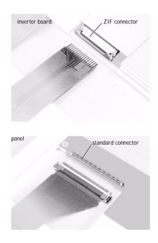
Replacing the Display Panel
