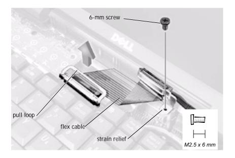
NOTICE: When reconnecting the flex cable, press down on both ends of the connector, not in the middle. Pressing the middle of the connector can damage fragile components.
