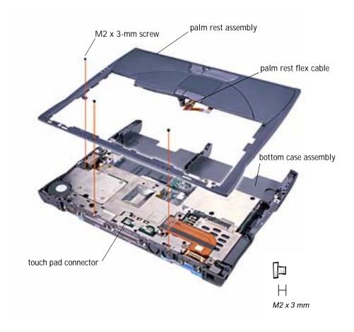
7 Using the plastic scribe along the edge of the plastic, remove the palm rest assembly from the bottom case assembly.
