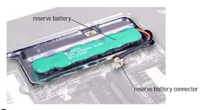
NOTICE: The reserve battery provides power to the computer's RTC and NVRAM when the computer is turned off. Removing the battery causes the computer to lose the date and time information as well as all user-specified parameters in the BIOS. If possible, make a copy of this information before you remove the reserve battery.
