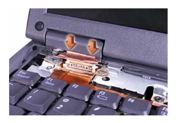
HINT: The right plastic hinge cover is labeled "R" and the left plastic hinge cover is labeled "L."
