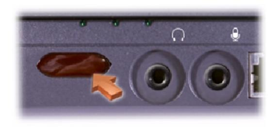
The infrared sensor lets you transfer files from your computer to another infrared-compatible device without using cable connections.
