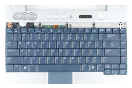
**7** Gently press the front of the keyboard down until the spring loaded tabs click into place and the keyboard is flat all the way across. The keyboard should easily fall into place. Be careful not to damage the LCD panel.
