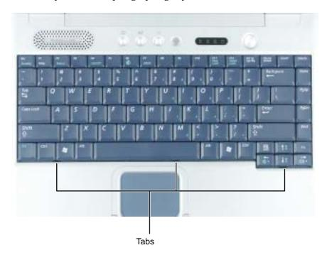
**12** While lifting the front of the keyboard, slide the keyboard toward you to release the five tabs at the back of the keyboard.
