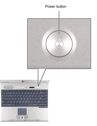
The power button is preset to On/Off mode. However, you can also set it to function in Standby/Resume mode. For instructions on changing the power button mode, see "Changing power settings" on page 153.
