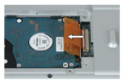
**9** Pry up on the left side of the hard drive (the side away from the connector) by inserting a flat-blade screw driver in the small groove in the plastic.
