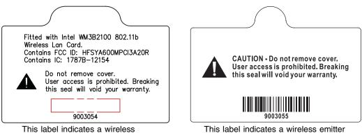
This label indicates a wireless emitter is installed in your notebook. This label indicates a wireless emitter is not installed in your notebook.
