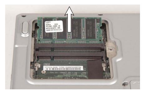
**8** If you are removing a memory module, pull the module out of the slot.
