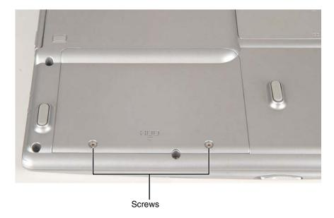
**6** Remove the two hard drive bay cover screws.
