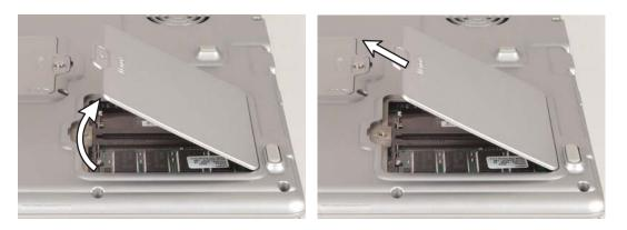
7 If you are removing a module, gently press outward on the clip at each end of the memory module until the module tilts upward.
