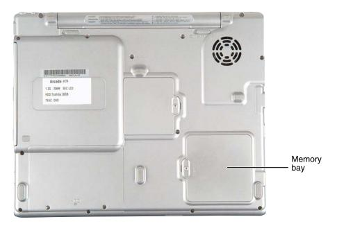
To add or replace memory modules: **1** Follow the instructions under "Preventing static electricity discharge" on page 226. **2** Turn off your notebook and disconnect the AC adapter and modem and network cables. **3** Turn your notebook over so the bottom is facing up. **4** Remove the battery. For more information, see "Replacing the battery" on page 149. **5** Loosen the memory bay cover screw. This screw cannot be removed. Screw
