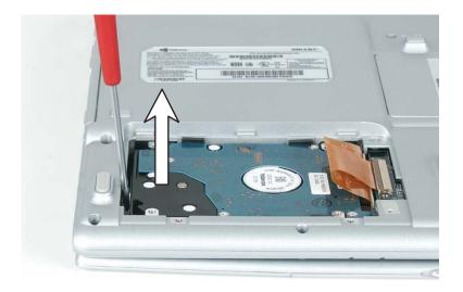
**10** Pull the hard drive away from the connector at a 45° angle and remove it from the notebook.
