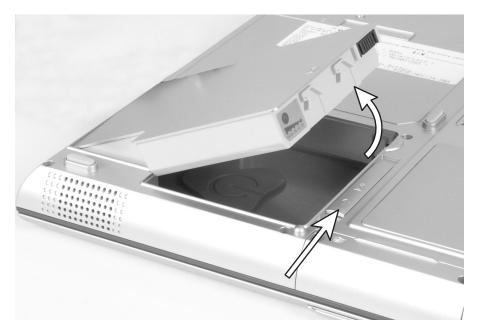
**4** Slide the battery release latch and lift the battery out of the bay.
