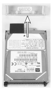
**10** Insert the new drive into the bracket so the screw holes line up and the plastic strip on the top of the bracket is positioned as shown.
