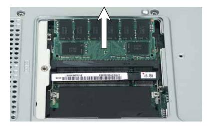
10 Hold the new or replacement module at a 30-degree angle and press it into the empty memory slot. This module is keyed so it can only be inserted in one direction. If the module does not fit, make sure that the notch in the module lines up with the tab in the memory bay.
