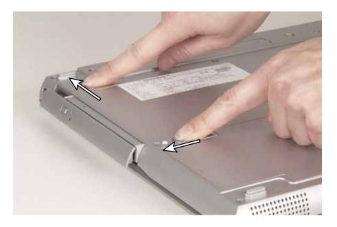
**7** Slide the other bay module release latch. The module moves out slightly.
