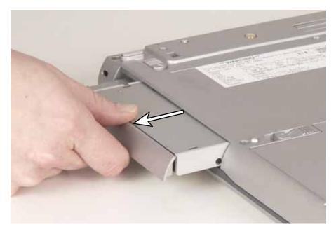
Firmly push the new bay module straight into the bay until the latches click into place.
