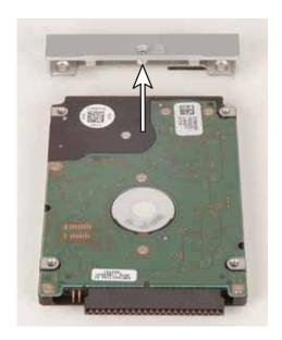
**12** Insert the new drive into the bracket so the screw holes line up and the plastic strip on the top of the bracket is positioned as shown.
