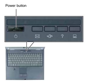
The power button is preset to On/Off mode. However, you can also set it to function in Standby/Resume mode. For instructions on changing the power button mode, see "Changing power settings" on page 163.
