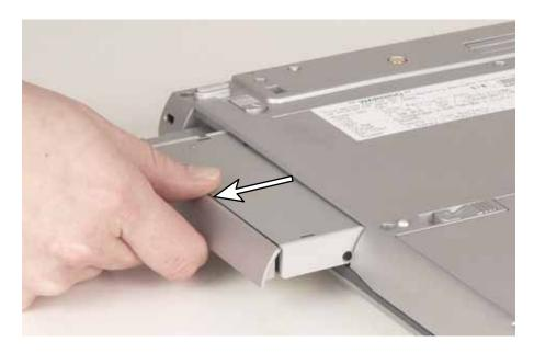
**9** Firmly push the secondary battery straight into the bay until the latches click into place.
