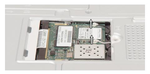
**9** Move the antenna wires out of the way, then press outward on the clip at each side of the module until the module tilts upward.
