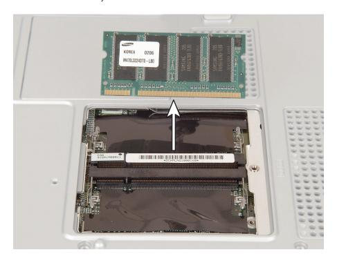
10 Hold the new or replacement module at a 30-degree angle and press it into the empty memory slot. This module is keyed so it can only be inserted in one direction. If the module does not fit, make sure that the notch in the module lines up with the tab in the memory slot.
