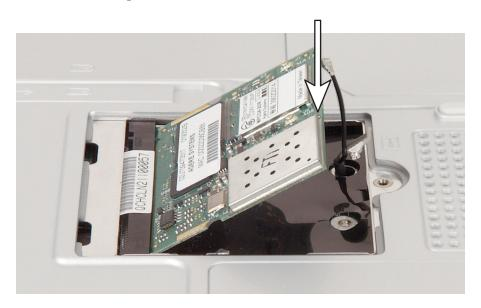
**13** Reattach the black antenna cable to the connector labelled MAIN or M, then reattach the light gray antenna cable to the connector labelled AUX or A.
