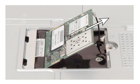
11 Hold the new module at a 30-degree angle and press it into the empty slot. This module is keyed so it can only be inserted in one direction. If the module does not fit, make sure that the notch in the module lines up with the tab in the module slot.
