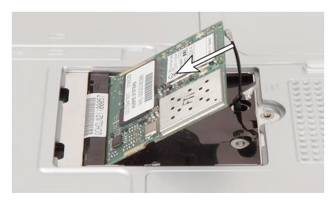
**12** Move the antenna wires out of the way, then press the module down until it clicks into place.
