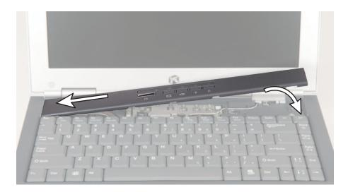
10 Press down on the cover in several places until it clicks in place. The cover is correctly mounted when you can run your finger along the cover and find no loose spots. The cover should be flat all the way across.
