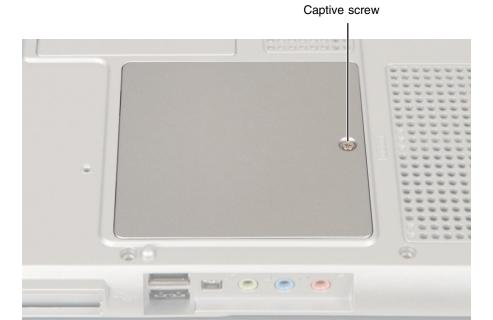
**6** Lift the screw side of the cover upward.
