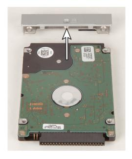
**8** Insert the new drive into the bracket so the screw holes line up and the plastic strip on the top of the bracket is positioned as shown.
