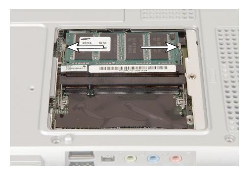
**9** Pull the memory module out of the slot.
