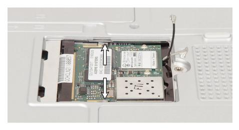
**10** Pull the module out of the slot.
