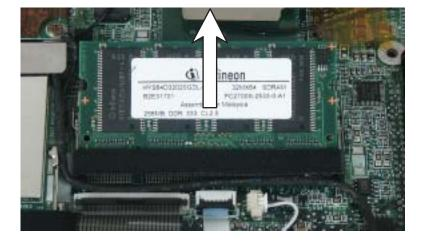
**3** Hold the new or replacement module at a 30-degree angle and press it into the empty memory slot. This module is keyed so it can only be inserted in one direction. If the module does not fit, make sure that the notch in the module lines up with the tab in the memory bay.
