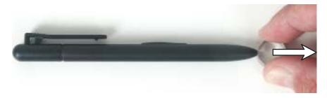
2 Insert a new point and apply slight pressure to set it in place.
