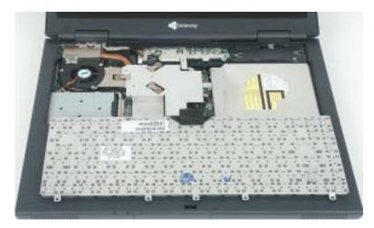
Pull up on the plastic keyboard connector using two fingers. After the connector is in the raised position, gently pull the cable out of the connector. Be careful not to touch or damage any other components.
