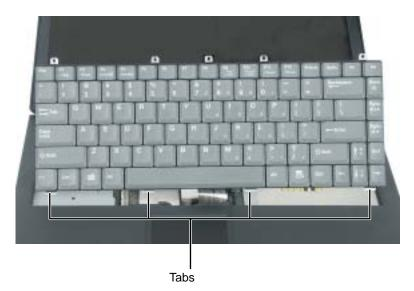
**7** Gently press the keyboard down until it is flat all the way across. The keyboard should easily fall into place. Be careful not to damage the LCD panel.
