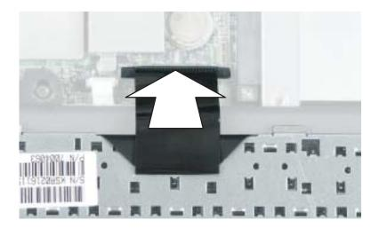
**5** Rotate the keyboard toward the LCD panel until the keyboard is almost face-up.
