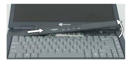
With a small Phillips screwdriver, remove the four keyboard screws and put them in a safe place.
