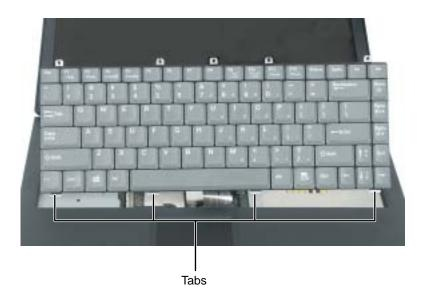
**3** Gently press the keyboard down until it is flat all the way across. The keyboard should easily fall into place. Be careful not to damage the LCD panel.
