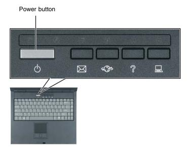
The power button is preset to On/Off mode. However, you can also set it to function in Standby/Resume mode. For instructions on changing the power button mode, see "Changing power settings" on page 157.
