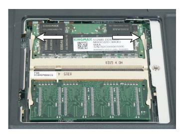
**7** Pull the memory module out of the slot.
