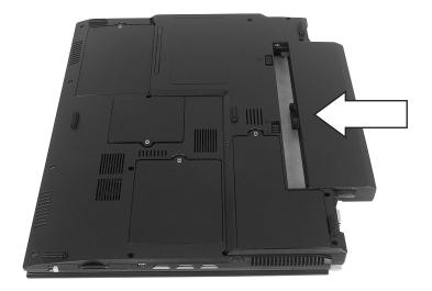
**4** Slide the battery lock to the locked position.
