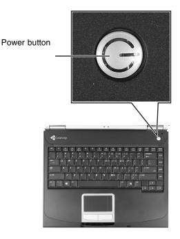
The power button is preset to On/Off mode. However, you can also set it to function in Standby/Resume mode.
