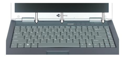
The bezel is correctly mounted when you can run you finger along the bezel and find no loose spots. The bezel should be flat all the way across.
