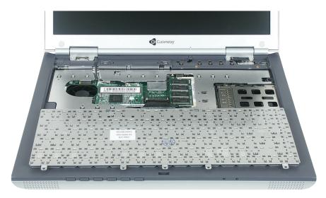
12 Carefully insert the small flat-blade screwdriver between the keyboard cable and the black plastic hinge where the cable connects to the system board. Gently lift the hinge off the cable. The cable is now free and you can remove the keyboard.
