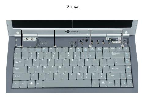
11 Lift the back edge of the keyboard, then slowly rotate it toward you so it lies **keys-down** on top of your notebook. Be careful not to damage the LCD panel.
