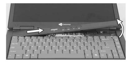
**10** With a small Phillips screwdriver, remove the four keyboard screws and put them in a safe place.
