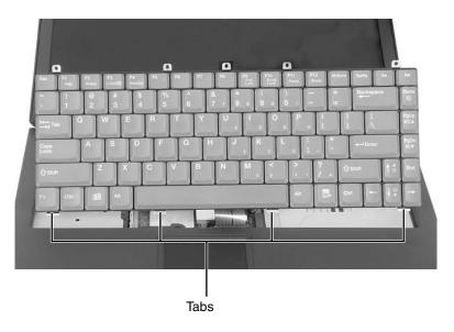
**2** Insert the tabs on the front of the keyboard under the palm rest.
