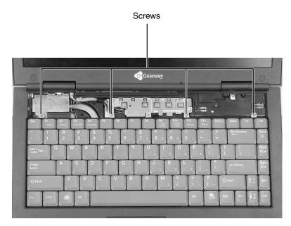
**11** Lift the back edge of the keyboard, then slowly rotate it toward you so it lies **keys-down** on top of your notebook. Be careful not to damage the LCD panel.
