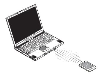
To use FIR, position two IR-aware devices so their IR ports are no more than one meter apart and offset no more than 15 degrees.
