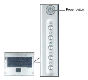
The power button is preset to On/Off mode. However, you can also set it to function in Standby/Resume mode. For instructions on changing the power button mode, see "Changing power settings" on page 152.
