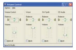
If the device you want to adjust does not appear in the window, click **Options**, **Properties**, the check box next to the audio device you want to adjust, then click **OK**.
