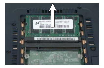
8 Hold the new or replacement module at a 30-degree angle and press it into the empty memory slot. This module is keyed so it can only be inserted in one direction. If the module does not fit, make sure that the notch in the module lines up with the tab in the memory bay.
