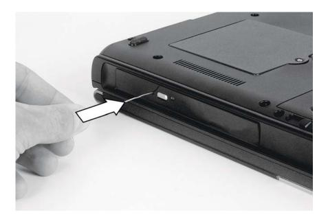
**9** Pull the drive tray open, then carefully slide the drive out of the drive bay.
