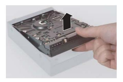
**9** Make sure that the jumpers on the new drive are set the same as the jumpers on the drive you are replacing.
