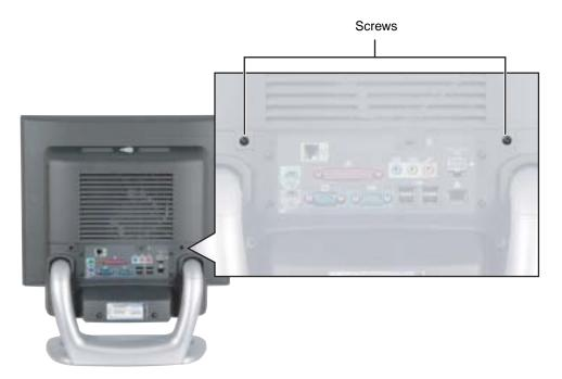
**3** With your hands positioned on each side of the case, swing the access panel up and away from the case and set the access panel aside.
