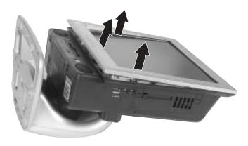
**5** Remove the four screws that hold the LCD panel to the case.
