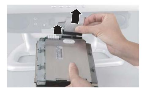
**5** Disconnect the diskette drive cable from the ZIF connector on the drive adapter card.
