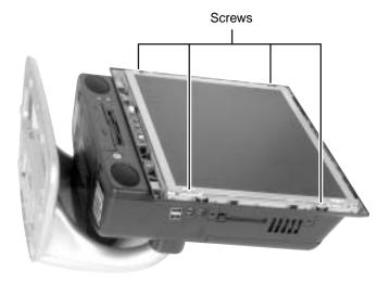
**6** Carefully tilt the bottom of the LCD panel slightly away from the case to access the cables behind the panel.
