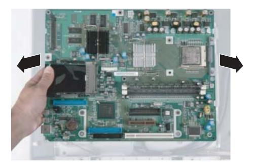
**32** Secure the new system board to the computer with the five screws removed in Step 30.
