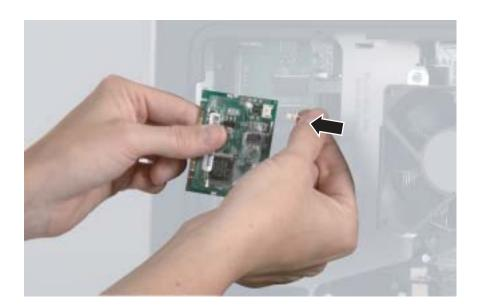
11 Carefully press the new Mini-PCI card into the card slot. The card must be fully seated in the slot before the retaining clips will snap into place.
