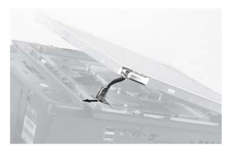
**8** Tilt the LCD panel up further and unplug the other cable from the inverter board, then unplug the scaler board connector from the LCD panel.
