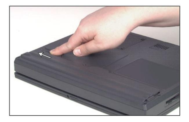
6. Hold the latch forward and lift the battery pack straight out from the notebook.
