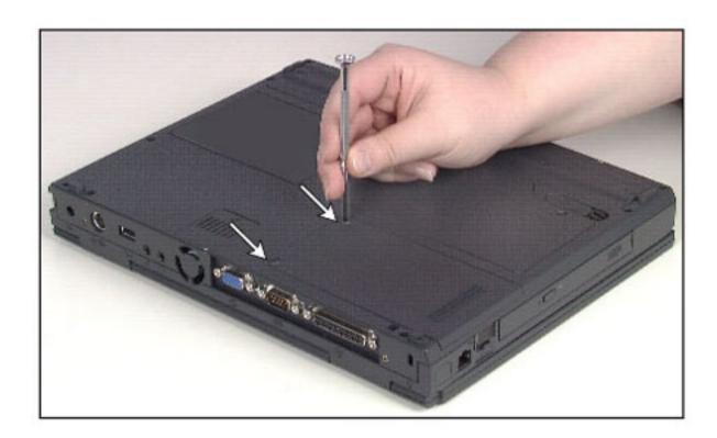
8. Slide the hard disk drive kit out and lift it up.
