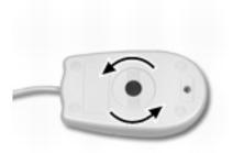
3. Remove the retaining ring and mouse ball.
