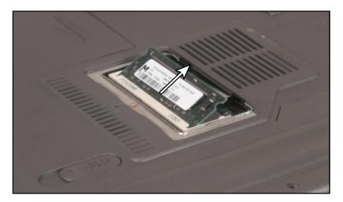
**7** Hold the replacement module at a 30-degree angle and press it into the empty memory slot. This module is keyed so that it can only be inserted in one direction. If the module does not fit, make sure the slot in the module lines up with the tab in the memory bay.
