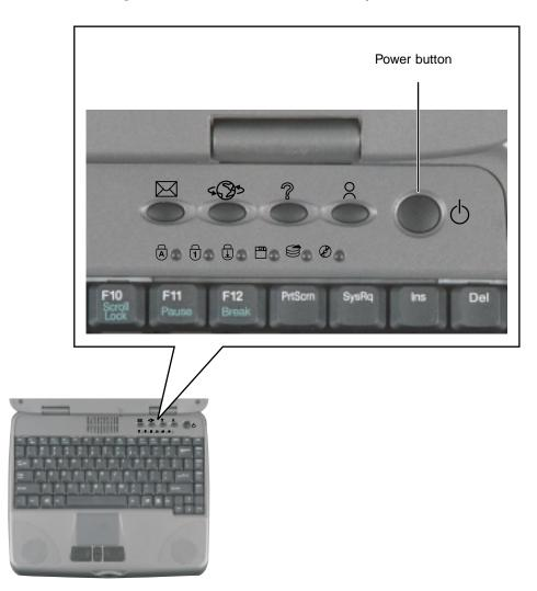
The power button is preset to On/Off mode. However, you can also set it to function in Standby/Resume mode. For instructions on changing the power button mode, see "Changing automatic power settings" on page 111.
