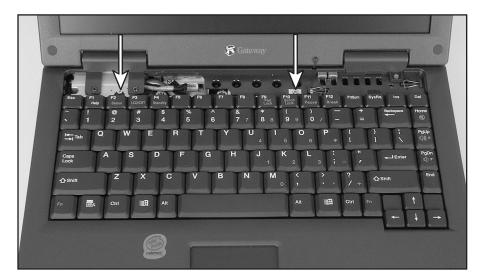
**9** Slide the two tabs located on the left end of the bezel under the notebook frame.
