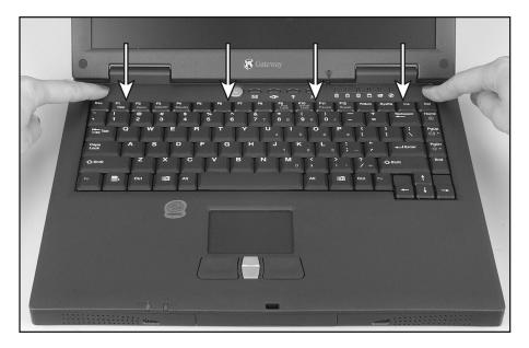
The bezel is correctly mounted when you can run you finger along the bezel and find no loose spots. The bezel should be flat all the way across. If the bezel is mounted incorrectly, complete the instructions under "Replacing the bezel" on page 11.
