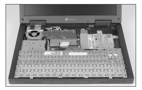
**11** Pull up on the plastic keyboard connector using two fingers. After the connector is in the raised position, gently pull the cable out of the connector. Be careful not to touch or damage any other components.
