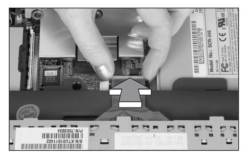
**5** Rotate the keyboard toward the LCD panel until the keyboard is almost face-up.
