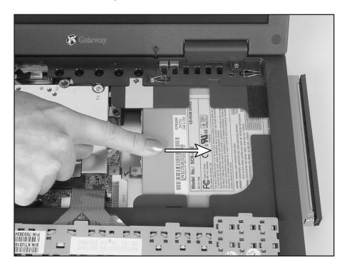
3 Slide the new drive into the same bay that the existing drive was located in. The drive is inserted properly when the logo on the drive door is right side up.
