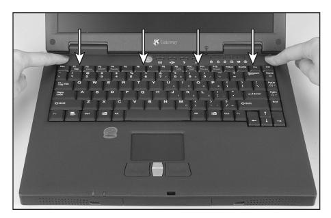
The bezel is correctly mounted when you can run you finger along the bezel and find no loose spots. The bezel should be flat all the way across. If the bezel is mounted incorrectly, complete the instructions under "Replacing the bezel" on page 15.
