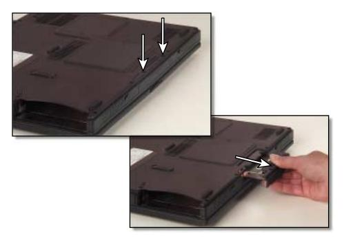
5 Place the new hard drive kit in the bay, slide it into the connector, then replace the screws to secure the hard drive to the notebook.
