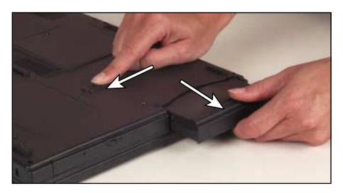
**3** Slide a charged battery into the bay until it snaps into place.
