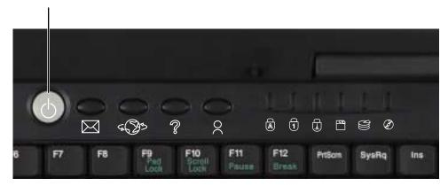
The power button is preset to On/Off mode. However, you can also set it to function in Standby/Resume mode. For instructions on changing the power button mode, see "Changing power settings" on page 99.
