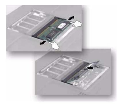
6 Hold the new or replacement module at a 30-degree angle and press it into the empty memory slot. This module is keyed so that it can only be inserted in one direction. If the module does not fit, make sure the notch in the module lines up with the tab in the memory bay.
