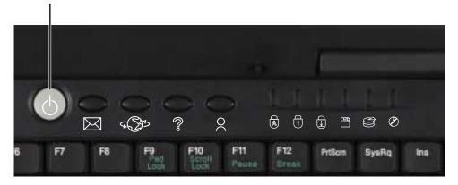
The power button is preset to On/Off mode. However, you can also set it to function in Standby/Resume mode. For instructions on changing the power button mode, see "Changing power settings" on page 137.
