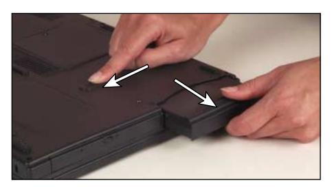
**4** Slide a new battery into the bay until it snaps into place.
