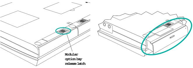
Figure 22. Locating the Release Latch (on the bottom of notebook)
