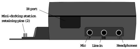
Figure 37. Mini-Docking Station - Left Side View
