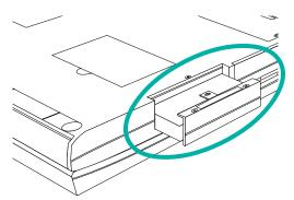
Figure 28. Removing the Hard Disk Drive
