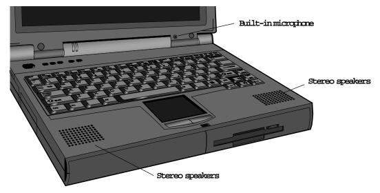
Figure 39. Locating the Built-in Speakers and Microphone
