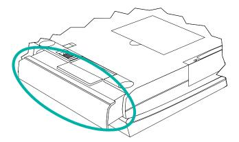
Figure 17. Removing the Battery Pack
