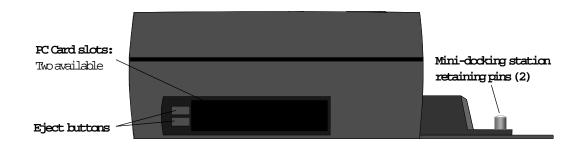
Figure 36. Mini-Docking Station - Right Side View
