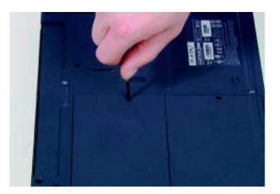
**7.** Slide the HDD out and lift up.
