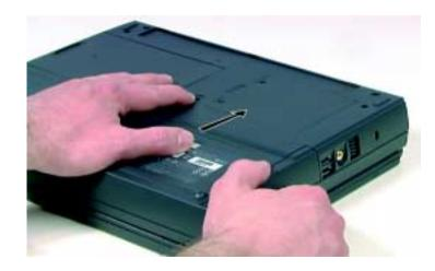
**5.** Hold the latch forward and slide the battery pack straight out from the notebook.
