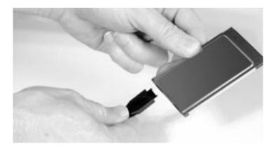
Plug the RJ11 connector into the XJACK connector as shown below:
