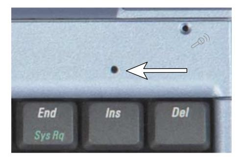
5 While pressing the paper clip down with your right hand, use your left hand to slide the bezel 1/8 inch (3.3 mm) to the left and remove the bezel and paper clip.
