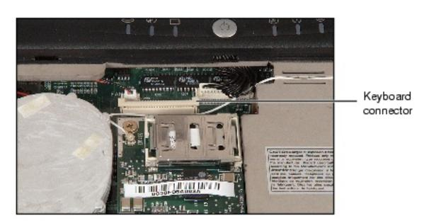
4. Slide the end of the keyboard cable into the keyboard connector.
