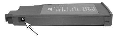
The battery begins charging, and the battery charge indicator turns red. When the battery is completely charged, the battery charge indicator turns off, and you can disconnect the AC power adapter.
