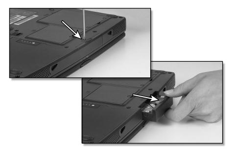
5 Place the new hard drive kit in the bay, slide it into the connector, then replace the screw to secure the hard drive to the notebook.
