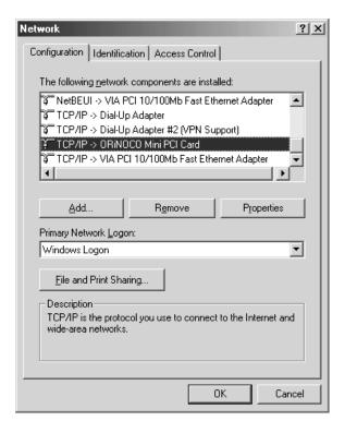
3 Select TCP/IP -> ORINOCO Mini PCI Card, then click Properties. The TCP/IP Properties dialog box opens.
