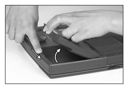
**3** Place a charged battery into the bay and press down until it snaps into place.
