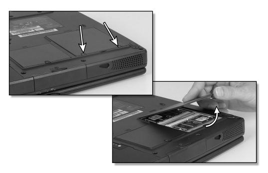
5 If you are removing a module, gently press outward on both clips at either end of the memory module until the module tilts upward. Pull the memory module out of the slot.
