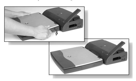
**5** Press down on the release latch until it snaps into place.
