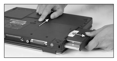
**3** Firmly push the second battery straight into the bay until the latch clicks into place.
