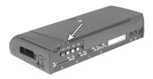
4 Lift the release latch on the docking station, then slide the cover straight back and lift it off.
