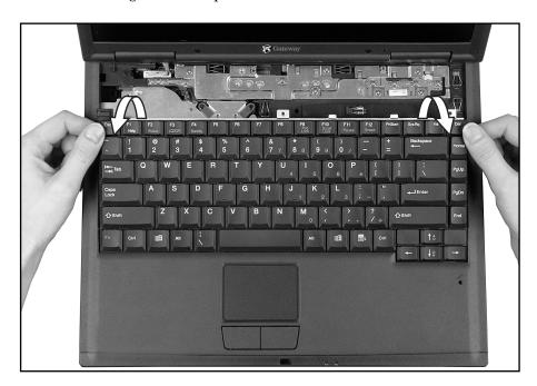
**9** Disconnect the keyboard by lifting the keyboard connector using two fingers. Be careful to not touch or damage any other components.
