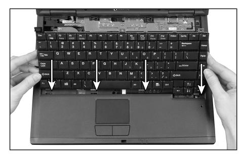
Gently press the keyboard down until it is flat all the way across. The keyboard should easily fall into place. Be careful to not damage the LCD panel.
