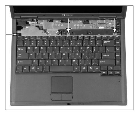
**8** Remove the keyboard by raising the back edge, then slowly rotating it toward you so it lies **keys-down** on top of the notebook. Be careful to not damage the LCD panel.
