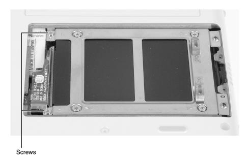
**8** Lift the end of the hard drive bracket nearest the edge of the tablet, then swing it toward the left until the bracket is laying on top of the tablet.
