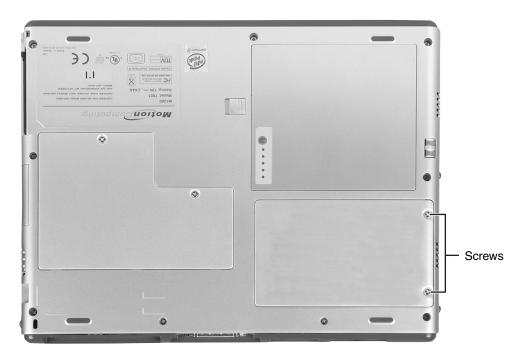
**7** Remove the two screws that secure the hard drive bracket to the tablet.
