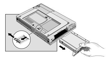
4. Slide the secondary battery into the module bay until it clicks into place.
