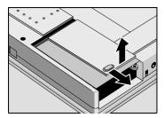
5. Insert the RAM board into the connector at about a  $30^\circ$  angle, then press down at both sides until it latches. Make sure it is properly seated.
