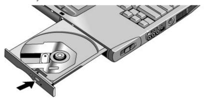
If your computer loses power, or if you have removed the CD-ROM or DVD module from the computer, you can manually open the drive to remove a CD. Insert a straightened paper clip into the recessed hole on the front of the drive to open it.
