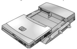
3. Position your fingers on the platform grips as shown below. Use your thumbs to push the computer into the dock until the computer slides into place.
