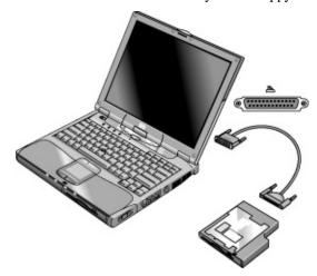
Before disconnecting the floppy disk drive, use the icon in the taskbar to stop the drive, or else shut down the computer. See "To replace a plug-in module" on page 76.
