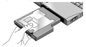
5. Slide the new plug-in module into the computer until it clicks into place.
