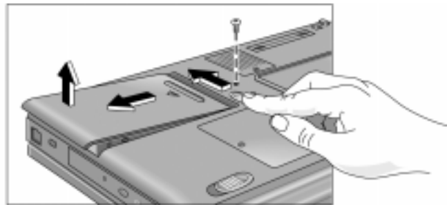
Figure 2-4. Removing the Hard Disk Drive
