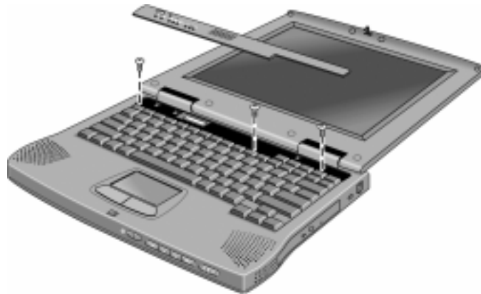
Figure 2-5. Removing the Keyboard Cover and Screws
